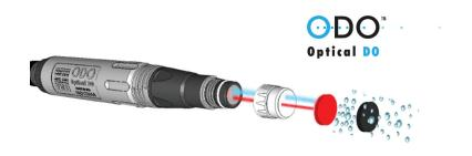
With optical DO, oxygen is constantly diffusing through the sensing cap affecting the luminescence of the sensing layer. The lifetime of the luminescence is measured by the sensor and compared against a reference.
